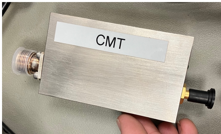
Figure 1. A ULNA from Cosmic Microwave Technology. The N Type connector on the left is the input, the SMA on the right is the RF output, as well as the input for DC bias and the calibrator control signal. A green indicator LED next to the SMA connector illuminates when the internal noise source is active.
