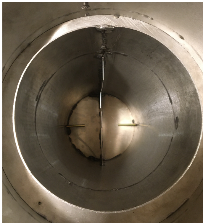
Figure 10. Input probes installed in the antenna
