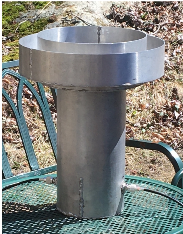
Figure 1. The compact circular septum feed under free-space test
