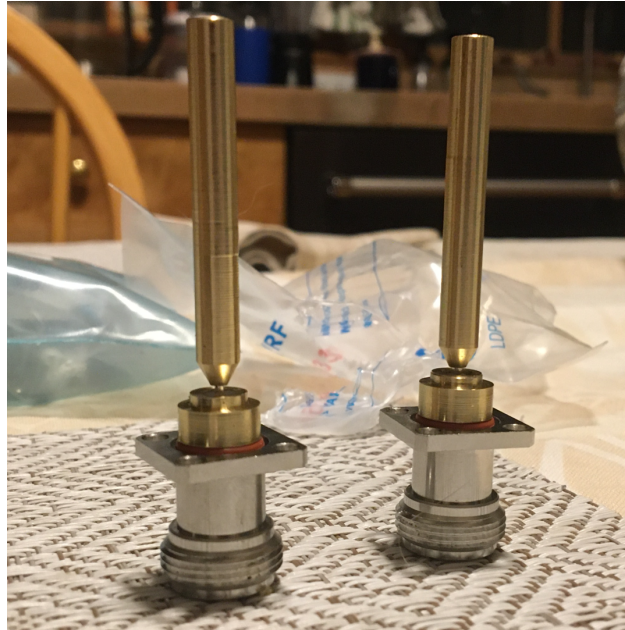
Figure 9. Completed input probe assemblies prior to insertion into the feed. Note that the choice of brass for the outer conductor sleeve was made for machining convenience for the prototype, and should probably be aluminum in future designs.
